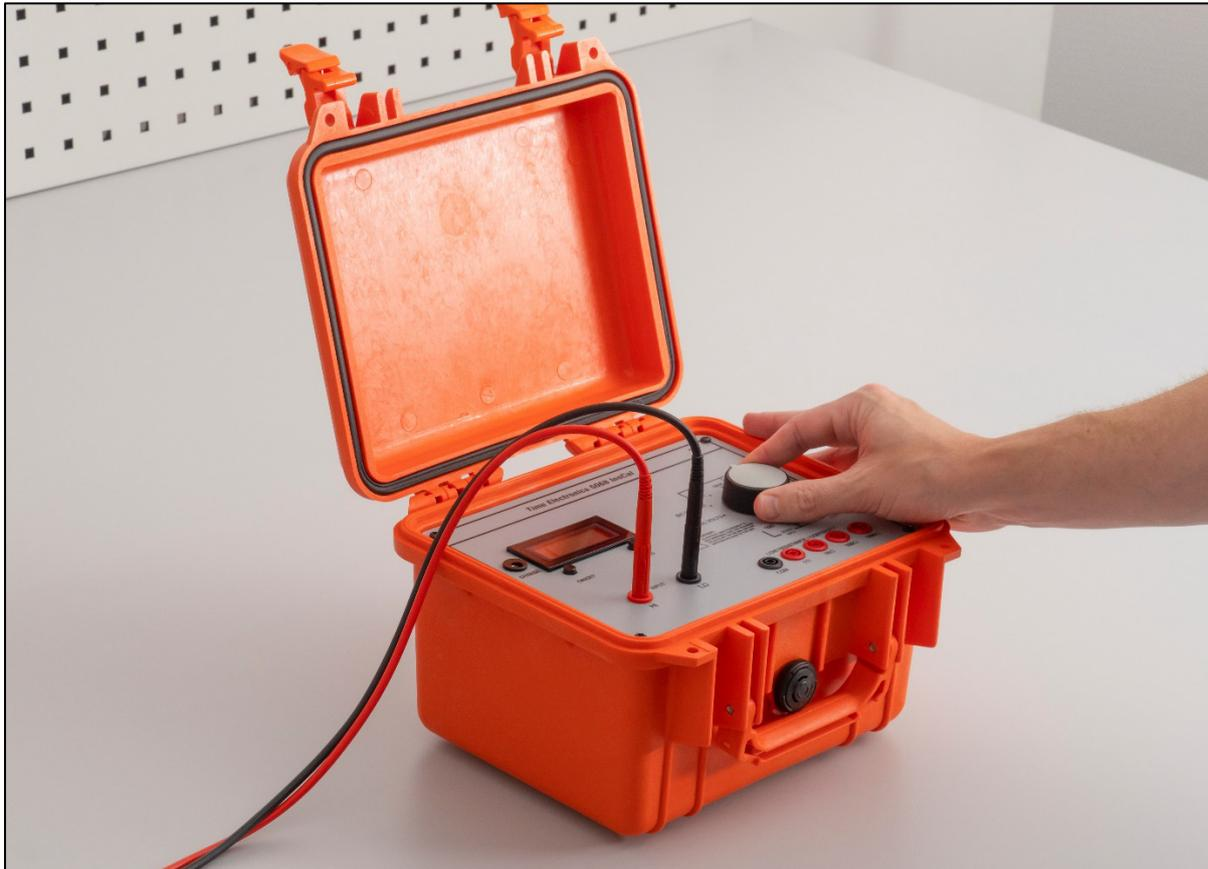
This 5068 provides all the equipment necessary to test and calibrate insulation test sets and megohm meters. It consists of:
